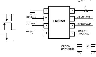
Fig. 2. Monostable Operation
