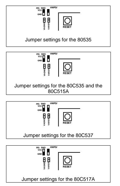
The other pin assignment differences, namely the VBB/VCC pin 37 of the 80535 family and the OWE input of the 80537 family of microcontrollers are addressed by jumpers on the respective daughter boards.
