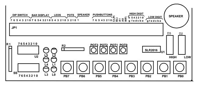
Figure 7.1 UIODs -- User Input/Output Devices
