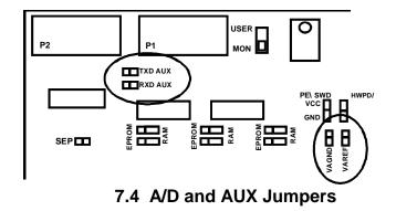
The jumpers TXD AUX and RXD AUX, when installed, connect the second serial port of the 80517 transmit and receive signals (P6.2 and P6.1) to the auxiliary serial port driver. If port bits P6.1 and P6.2 are to be used as general purpose input/output ports, these jumpers should be removed.
