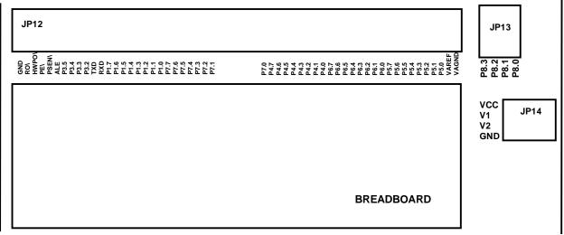
Figure 7.2 JP12, Microcontroller Ports
