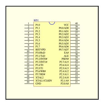
Figure 1.1. Pinout of the 8051 Microcontroller (NC stands for No Connection).
