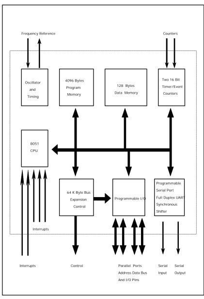
Figure 1.2. The Block Diagram of the 8051 Microcontroller.
