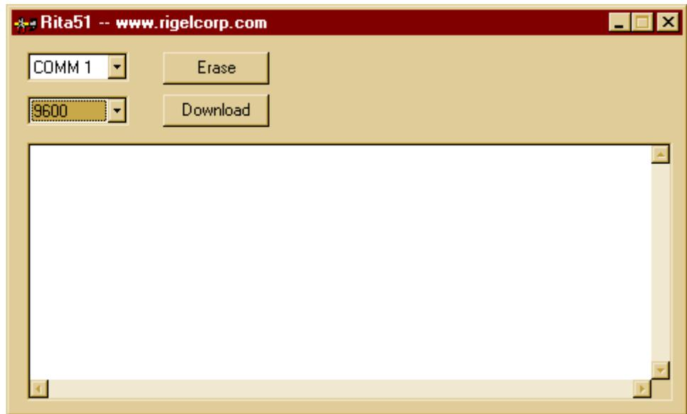
The Rita-51 Utility has two buttons. The "Erase" button erases the FLASH ROM. The "Download" button asks for a program file in the Intel hex format. It opens and downloads the file to the board. Once you download your program, move the slide switch to the RUN position and press the reset push button. Your code in FLASH ROM now constitutes the 8051 code memory. The RAM is mapped into the 8051 external data (XDATA) memory.
