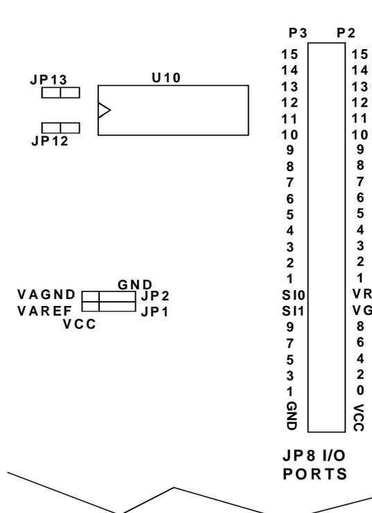
Figure 4.2 Serial Port and A/D Jumpers
