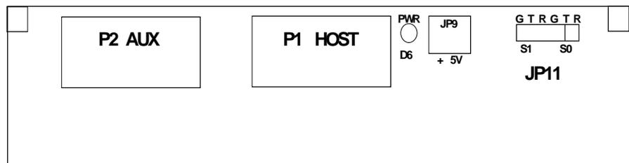
Figure 3.2 Serial Port Connectors
